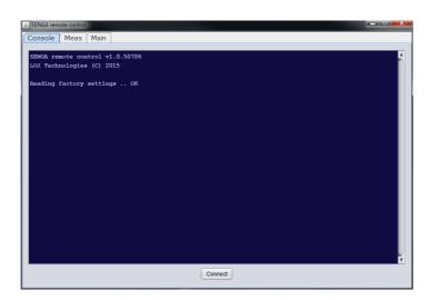
Console panel shows information about serial connection synchronization with SENGA devices. CONNECT/DISCONNECT button at bottom of the panel allows to start or stop connection session with all SENGA devices found at one of the existing serial ports.
