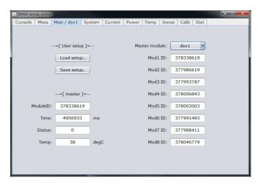
Main panel enables to load or store settings for all connected SENGA devices, and selection of SENGA module of user focus.
